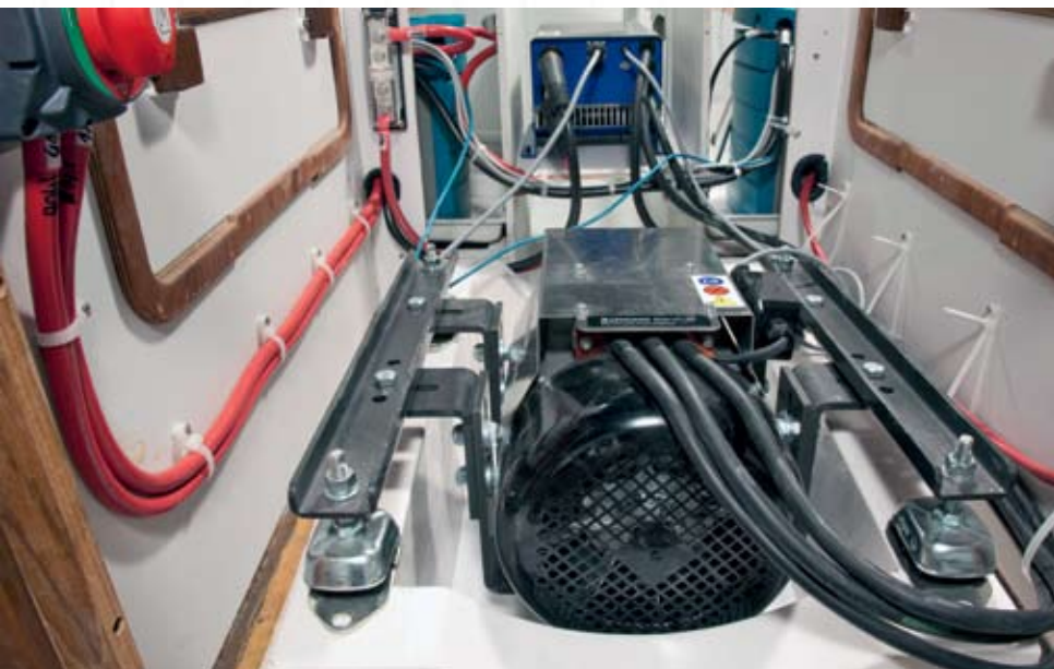
The boat is fitted with a 7.5kW Bellmann electric motor, mounted within a standard sail drive bed. Together with the lithium-ion technology, it offers near silent running for 3-4 hours at 6-7 knots.
